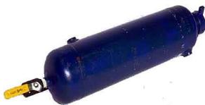
Best for SWAM® Automated Systems, the **Model 2B Air Dryer** offers a capacity of 13 SCFM at 100 psi (368 liters per minute at 7kg/cm<sup>2</sup>). The Model 2B Air Dryer holds 25 pounds of Super-Dry Tablet Desiccant that is capable of producing a 30°F dew point suppression.
