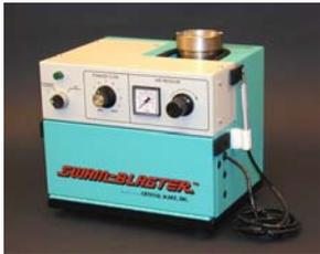
The unique design of the **Model MV-2 Micro Abrasive Blaster** and the **Model MV-2L** offers “Maximum Versatility” with carbide lined fittings throughout the abrasive pathway and with the tilting powder tank that is mounted to a hinged plate to allow it to tilt to the side and with the push of a button, the vibrator activates to simply walk the powder out for rapid powder changes.
