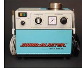
The **Model LV-1 (Large Volume) Micro Abrasive Blaster** is best for operating in production lines and in the SWAM® Automated Systems. The Model LV-1 features an hour meter for SPC monitoring and a leak detection system for the pinch valve assemblies. It holds approximately 20 pounds of aluminum oxide and has a separate mixing powder tank for a consistent powder feed rate from a full tank to an empty tank.
