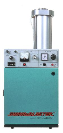
The **Model LV-1 (Large Volume)** is best for operating in production lines and in the SWAM® Automated Systems. The LV-1 features independently adjustable powder flow control and air pressure regulation for total process control, an hour meter for SPC monitoring and a leak detection system for the pinch valve assemblies. It holds approximately 20 pounds of aluminum oxide and has a separate mixing powder tank for a consistent powder feed rate from a full tank to an empty tank.
