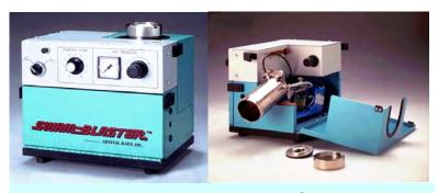
The unique design of all the *SWAM-Blaster* MV Series Micro Abrasive Blasters offers "Maximum Versatility" with carbide lined fittings throughout the abrasive pathway, the <u>tilting powder tank</u> is mounted to a hinged plate to allow it to tilt to the side and with the push of a button the vibrator activates to simply walk the powder out for <u>rapid powder changes</u>.
